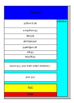
Fig. 3: Structure of the Self Extracting Executable
