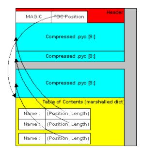
Fig. 1: Structure of the ZlibArchive
